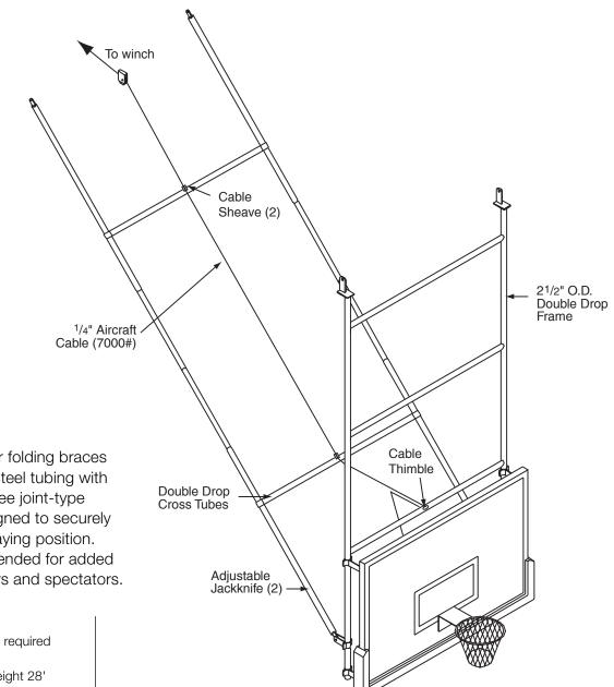
Fully adjustable rear folding braces are constructed of steel tubing with a jackknife-style, knee joint-type folding system designed to securely hold backstop in playing position. Safety belt recommended for added protection for players and spectators.
